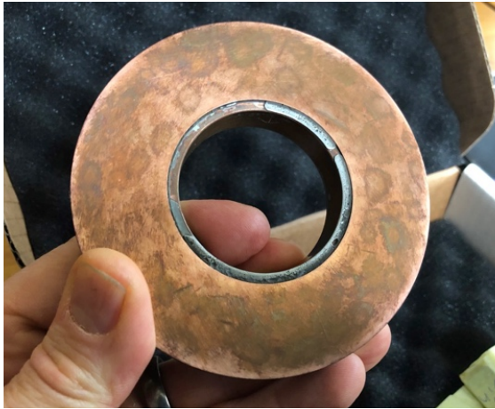
Fig. 4. Small HTS magnet manufactured by Tokamak Energy
