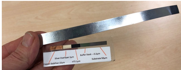
Fig. 2. High Temperature Superconductor tape sample
